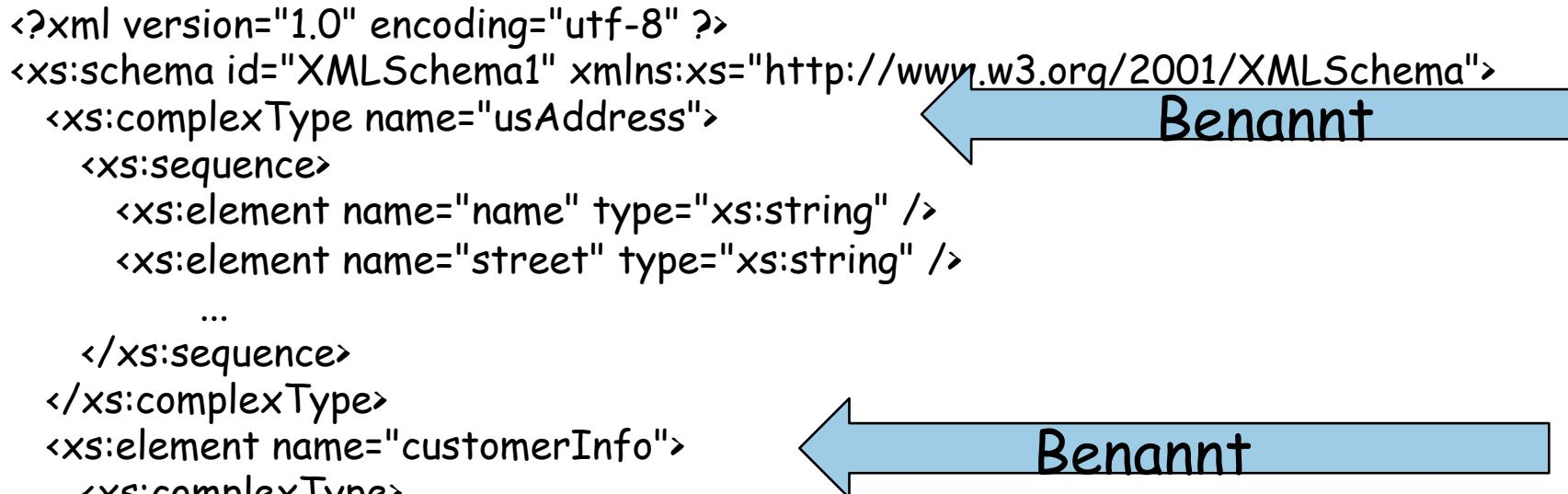
The diagram illustrates the concept of named types in XML Schema. It shows two specific elements from the schema: 'usAddress' and 'customerInfo'. Each element is preceded by a blue arrow pointing from the right towards the element definition. Above the first arrow, the word 'Benannt' is written, indicating that the 'usAddress' type is explicitly named. Below the second arrow, the word 'Benannt' is also written, indicating that the 'customerInfo' element is explicitly named.
